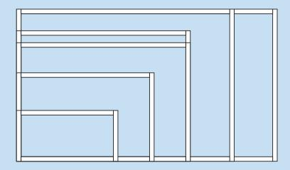
42" x 72" 42" x 60" 36" x 48" 32" x 48" 24" x 36" 14" x 38" Mounting options available in both horizontal and vertical orientations, frames are available in six standard sizes with the added flexibility to build to your specifications.
